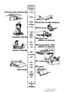
dB is the abbreviation for decibel - a unit of sound measurement. It is equivalent to 10 times the logarithm (to base 10) of the ratio of a given sound pressure to a reference pressure.
