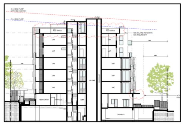
Figure 2: Section demonstrating no new works exceeding the maximum HOB (Source: Zhinar Architects)
