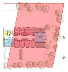
Figure 1: Proposed first floor plan, extent of rear 25% of subject site outlined in red hatching (Source: Team 2 Architects
