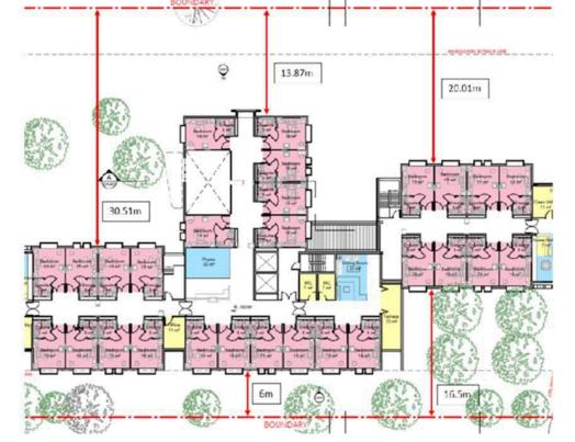
Figure 13: Proposed setbacks at first floor level (Source: Team 2 Architects)
