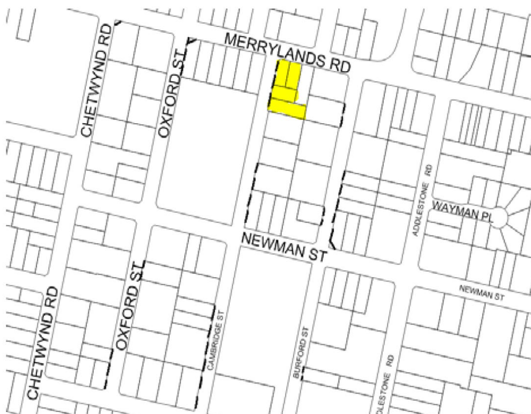
Figure 2 – DCP Provision for 1.5m Road Widening along Cambridge Street
