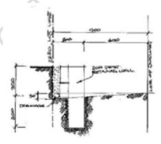
Figure 35: Retaining walls within maintenance easement
