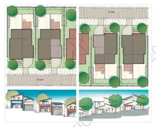
Figure 27: Split level house designs for cross slopes
