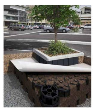
Example of using strata cells around hard surfaces (Photo courtesy of greenblue.com)
