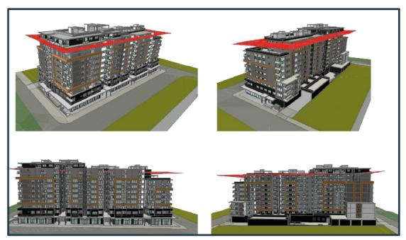
Figure 1: 3D Height Plane demonstrating the proposed exceedance of the building height control
