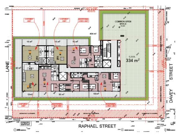
Figure 7: The north facing roof top terrace is complaint with the ADG requirements and the proposed addition is setback so that it does not add bulk and scale when viewed from the streetscape. The additional apartments provides casual surveillance and benefit from better outlook and amenity.
