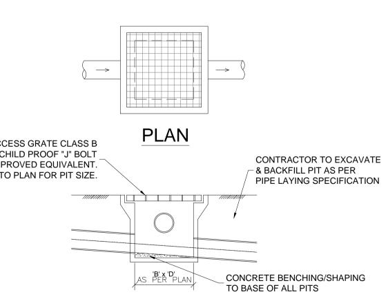
SECTION TYPICAL SURFACE INLET PIT TYPICAL FOR ALL PITS IN NON-TRAFFIC AREAS
